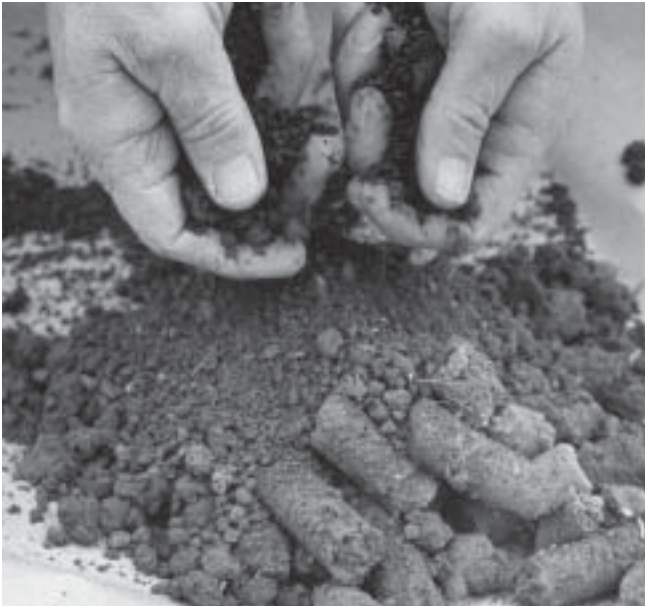
Figure 4. Break up clods while a sample is moist, and spread out to air dry in a clean area.
